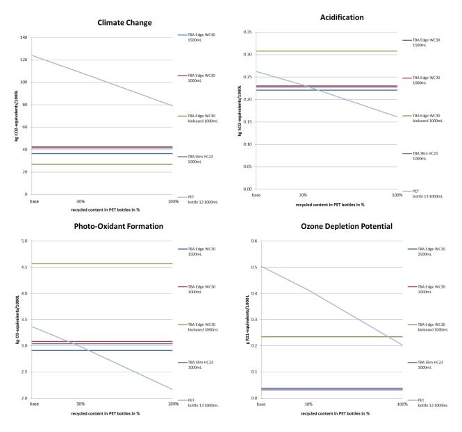
Figure 145: Indicator results for sensitivity analysis recycled PET of segment SD Family Pack, Switzerland, allocation factor 50% (Part 1)
