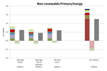
Figure 95: Indicator results for base scenarios with base collection quota of beverage cartons of segment JN FAMILY PACK, Switzerland, allocation factor 50% (Part 3)
