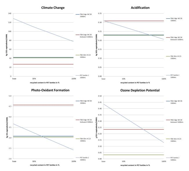
Figure 139: Indicator results for sensitivity analysis recycled PET of segment JN Family Pack, Switzerland, allocation factor 50% (Part 1)
