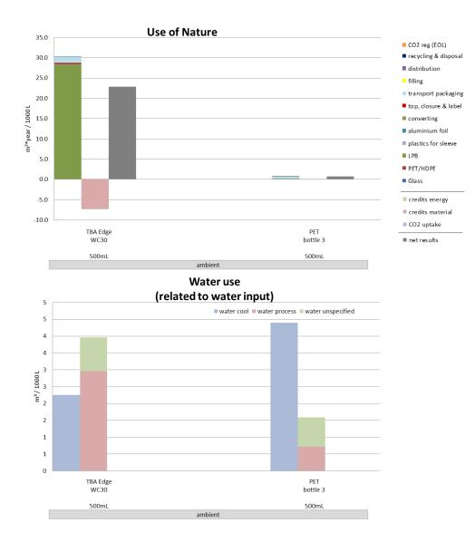
Figure 124: Indicator results for base scenarios with target collection quota of beverage cartons of segment SD PORTION PACK, Switzerland, allocation factor 50% (Part 4)
