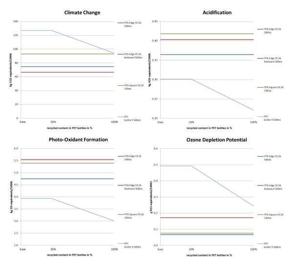
Figure 74: Indicator results for sensitivity analysis recycled PET of segment SD Portion Pack, Austria, allocation factor 50% (Part 1)
