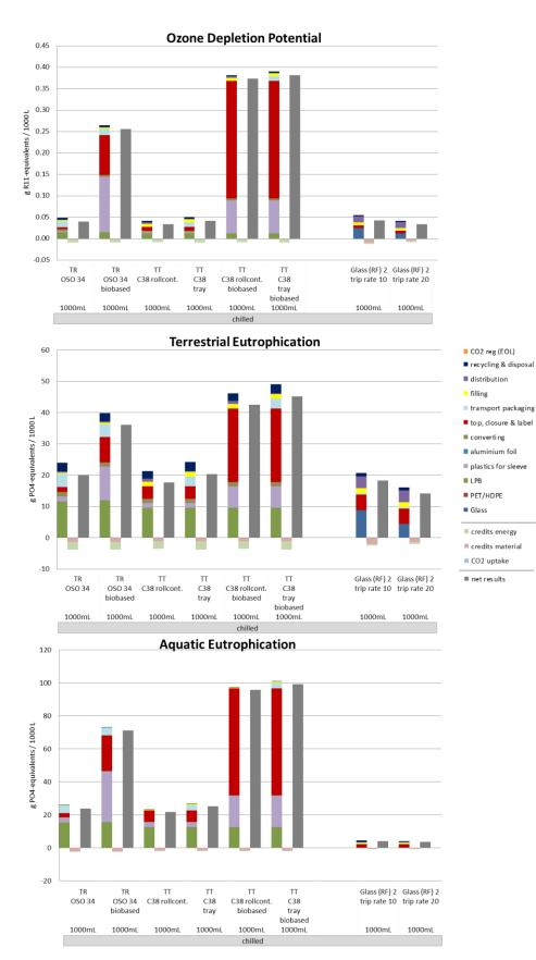
Figure 51 Indicator results for sensitivity analysis regarding trip rates of refillable glass bottles of segment DAIRY FAMILY PACK, Austria, allocation factor 50% (Part 2)
