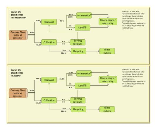
Figure 16: Applied average end-of-life quotas for one way glass bottles in Switzerland and Austria. Numbers in bold print represent the share on total mass flow, those in italics illustrate the share on the specific process.
