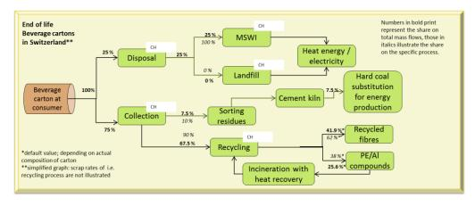
**Figure 12:** Applied target end-of-life quotas for beverage cartons in Switzerland. Numbers in bold print represent the share on total mass flow, those in italics illustrate the share on the specific process.
