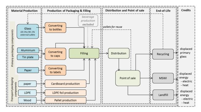
Figure 5: System boundaries of glass bottles one way
