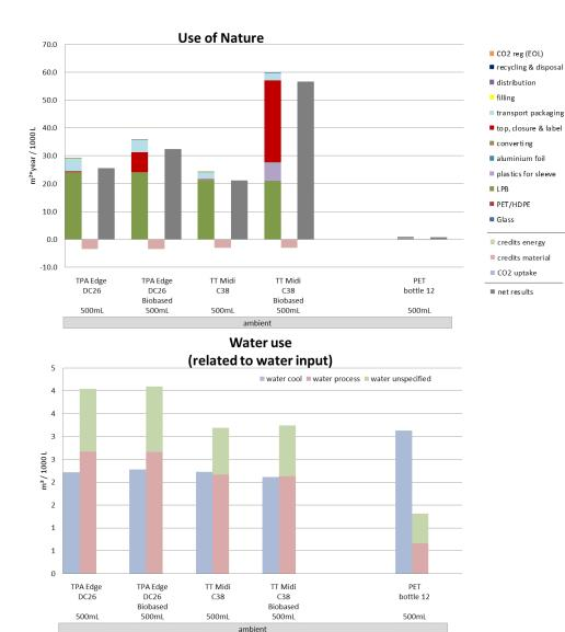
Figure 44: Indicator results for base scenarios of segment WATER PORTION PACK, Austria, allocation factor 50% (Part 4)
