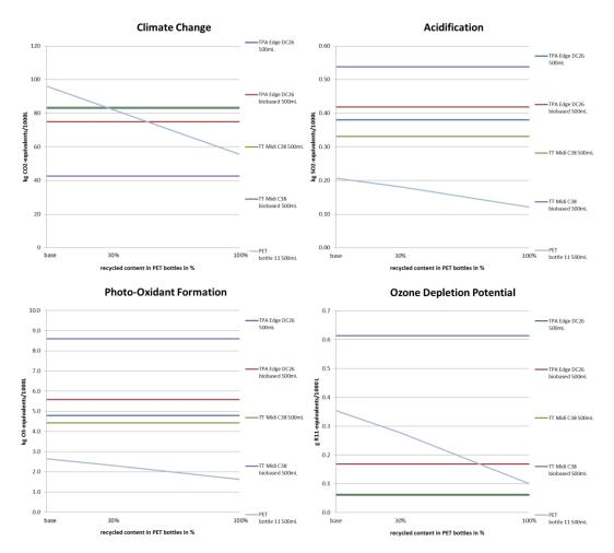
Figure 156: Indicator results for sensitivity analysis recycled PET of segment WATER Portion Pack, Switzerland, allocation factor 50% (Part 1)
